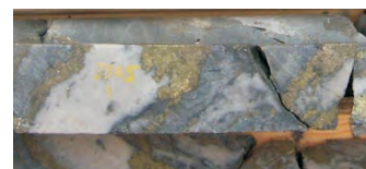
Brecciated and quartz veined volcanic rocks with abundant arsenopyrite, chalcopyrite, sphalerite and tetrahedrite. Specimen from 1.57 metre interval @ 2.03 g/t gold, 209 g/t silver, 1.81% copper (drill hole SH11-12 at 232.5m)
